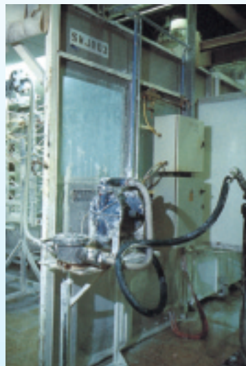
This Blagdon 25 metallic pump at Caradon Bathroom is feeding a robotic spray glazing operation.
